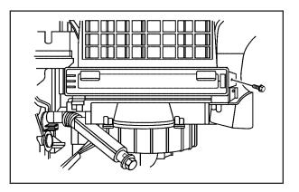
4. Remove the air filter cover screw.
